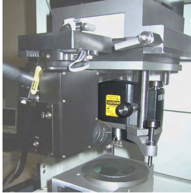
Fig. 5. UNMT with the AFM head and optical digital microscope attachments
